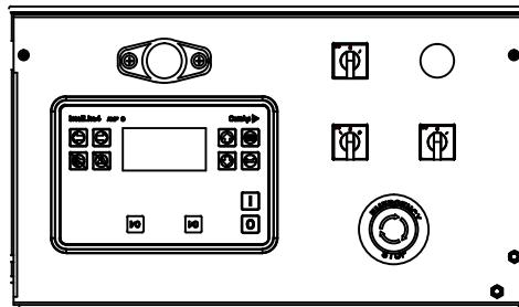
InteliLite4-AMF9 is Single Gen-set controller for stand-by and prime-power applications and all-in-one intuitive & powerful PC tool for configuration/monitoring/control, locally or remotely and easy to install, configure and use
