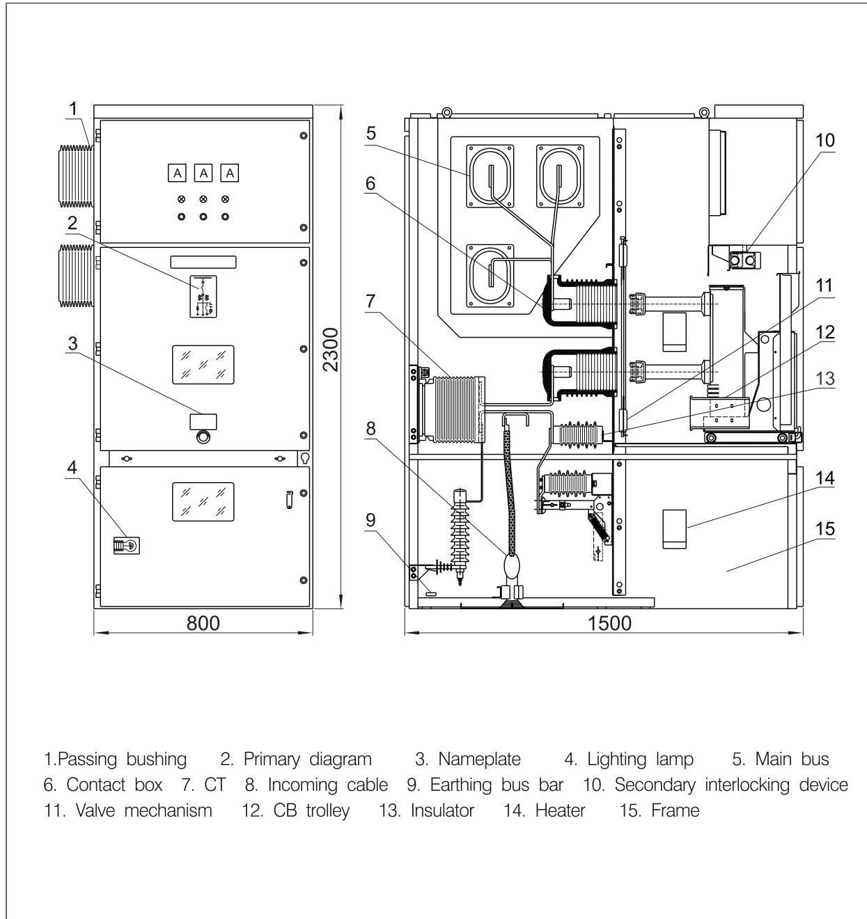
1. Passing bushing    2. Primary diagram    3. Nameplate    4. Lighting lamp    5. Main bus
