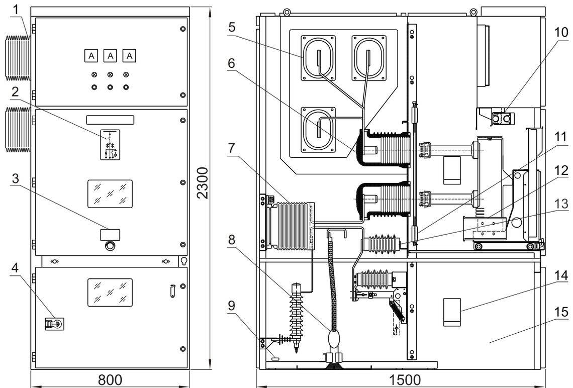
1. Passing bushing    2. Primary diagram    3. Nameplate    4. Lighting lamp    5. Main bus
