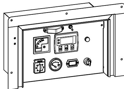
PLC-920 is an advanced control module based on micro-processor designed to control the engine via a key switch and push buttons on the front panel. The module is used to start and stop the engine and indicate fault conditions, automatically shutting down the engine and giving a true first up fault condition of an engine failure.
