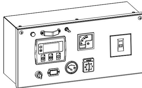
PLC-920 is an advanced control module based on microprocessor designed to control the engine via push buttons on the front panel. The module is used to start and stop the engine and indicate fault conditions, automatically shutting down the engine and giving a true first up fault condition of an engine failure.
