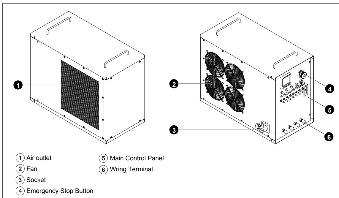
**Resistive Load Bank****Control Panel**
